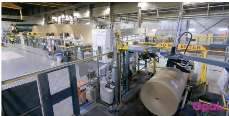
Opal cuts down its 50-tonne product into customer rolls through its winder, which range from 600mm wide, all the way to 2.8m wide.
