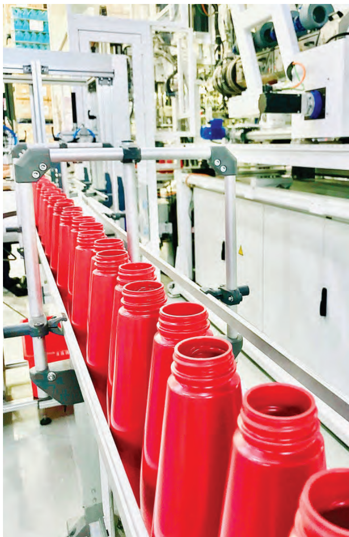
Production line for Wellman Packaging's Squeezy Sauce bottle, made from 90% food grade rPE.
