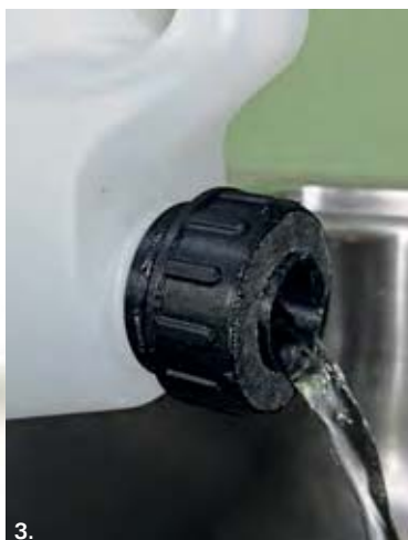
Caps and Closures' 38mm twist-and-pour cap at three stages of the design process: 1. Solidworks CAD Assembly 2. Rendered image and 3. 3D Printed Functional Part.
