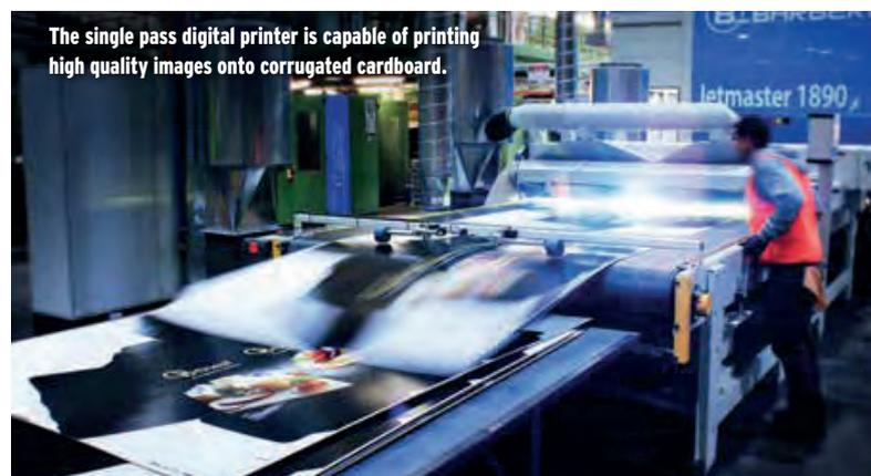
The single pass digital printer is capable of printing high quality images onto corrugated cardboard.
